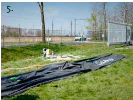
5. The SLAMDAM® now lies empty in the longitudinal direction.
